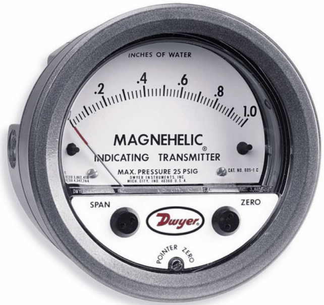
Figure 4. Pressure gauges measure static pressure inside poultry houses.
