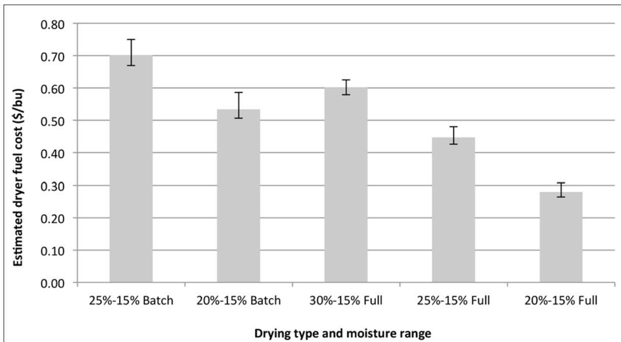
Figure 1. Estimated drying fuel cost by drying case (\$3/gal LP).
