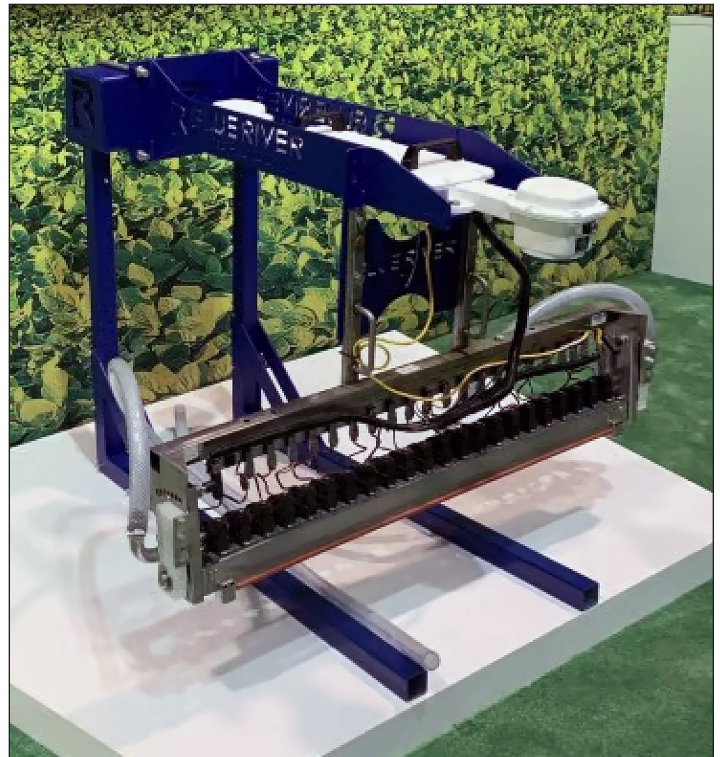
Figure 1. John Deere showed a See & Spray™ model from Blue River that will be used to target weeds with herbicides using artificial intelligence and precise spraying (Hamblen 2020).
