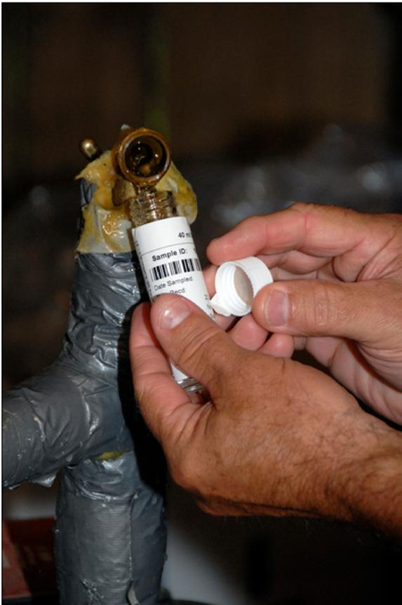
Figure 3. Use only the container provided by the testing laboratory for taking well-water samples.
