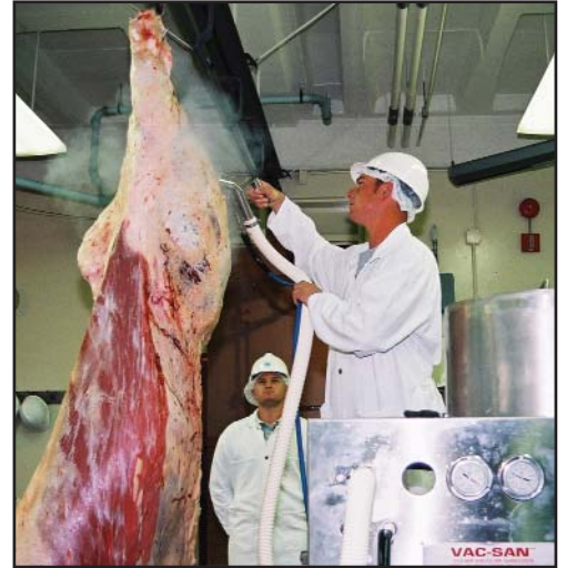
One way to reduce the incidence of E. coli 0157:H7 is to steam vacuum carcasses.
