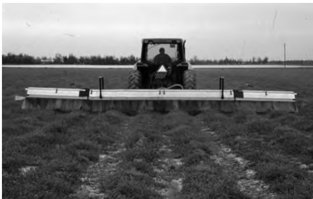
Figure 6. Broadcast shielded sprayer operating in "burn-down"
